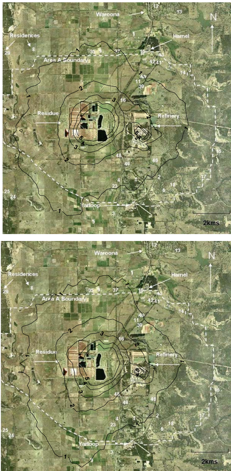
Figure 1: Average (99.5th percentile) acetaldehyde 3 minute concentrations ( \mu\text{g}/\text{m}^3 ) (data assimilated) for the existing (top) and expanded refinery (bottom)
