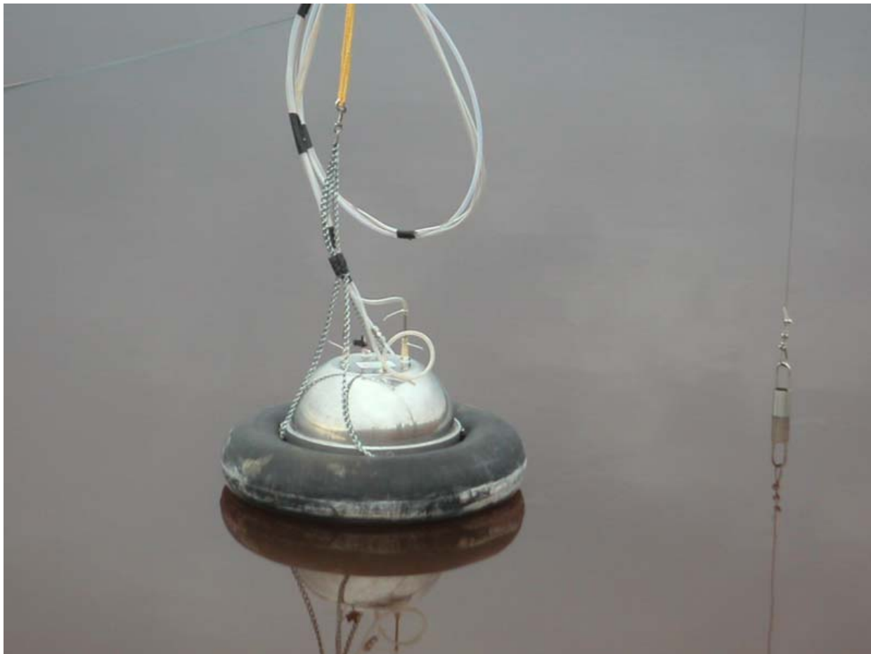
Figure 2. Flux Hood Floating on ROWS pond.
