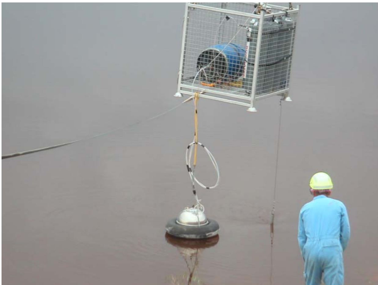
Figure 3. Sampling hood connected to Automated Sampling system
