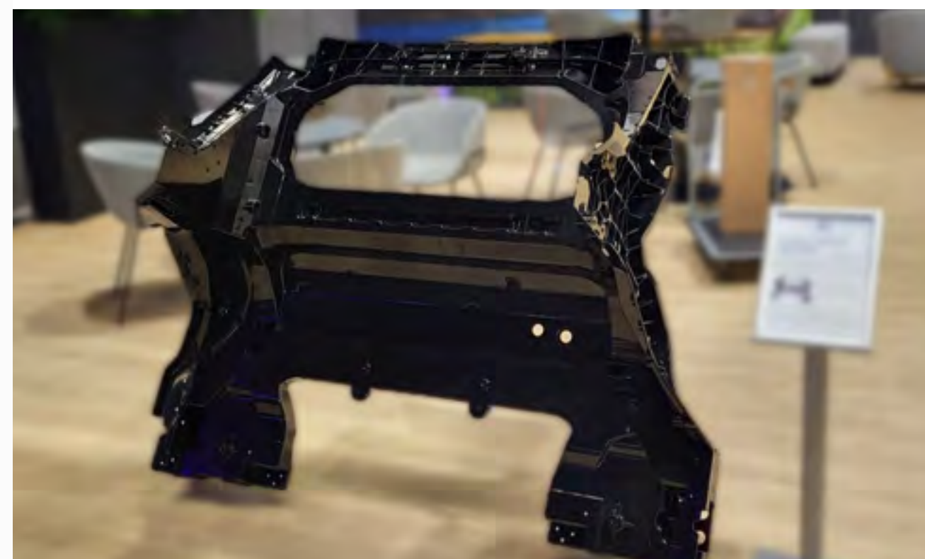
This rear floor frame megacasting for electric vehicle manufacturer NIO used our C611 EZCast™ alloy.
